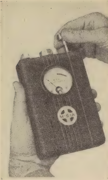
Courtesy Mine Safety Appliances Co. Fig. 123. Explosimeter used to determine combustible gas hazards.
