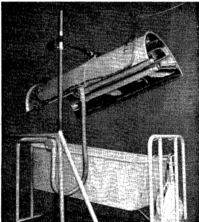
Fig. 6—Artificial-light apparatus for cradle illumination of infants.
