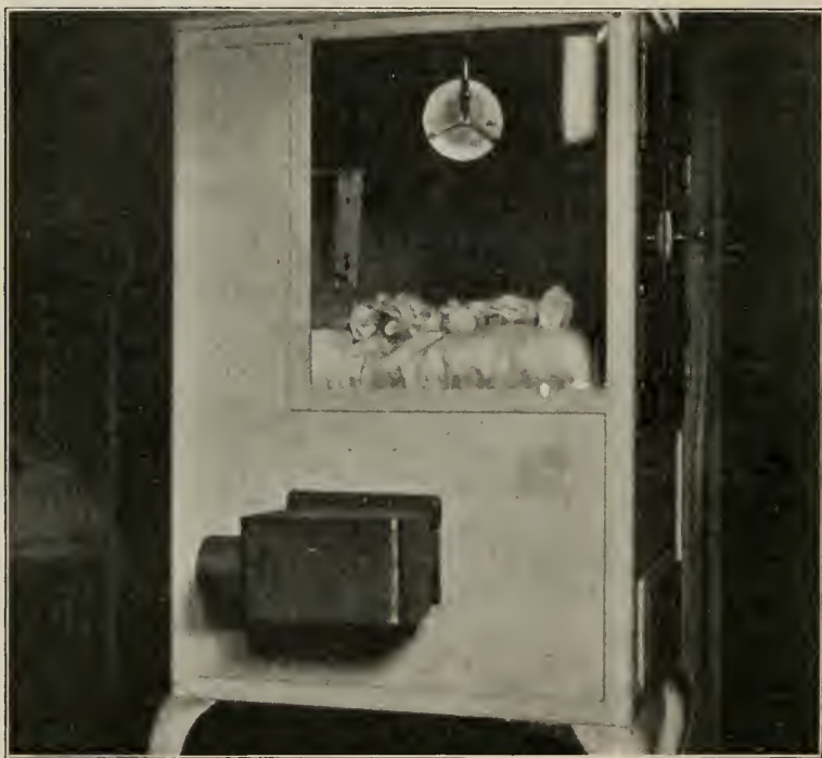
FIG. 5. — Showing Metal Box attached to the side of the Incubator into which the Air enters.
